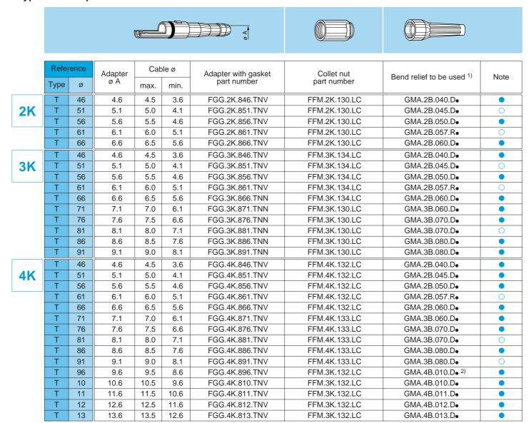
Note: 1) The bend relief is to be ordered separately (see pages 91 and 92). 2) Add a short piece of heat-shrink tubing under the bend relief.
