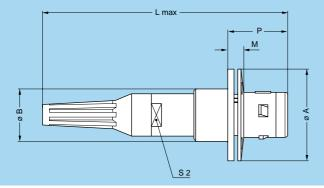
FMG Fixed plug with round flange, four hole fixing, key (G) or keys (A...F, L and R), cable adapter and nut for fitting a bend relief
