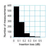
Mean = 0.10 dBTested at 1300 nm Tested according to the standard IEC 61300-03-04, Insertion Method B. Fibre =  $9/125 \mu m$ Ferrule bore diameter = 125 µm
