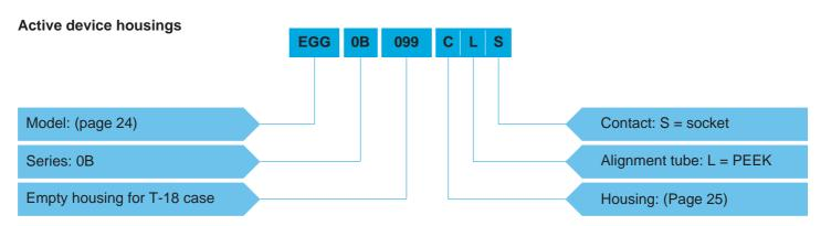
**EGG.0B.099.CLS** = Fixed active device housing, nut fixing, with key (G), 0B series, empty housing for TO-18 case, chrome-plated brass housing, PEEK alignment tube, socket contact.
