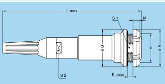
PEG Fixed socket, nut fixing, key (G) or keys (A...F, L and R), cable adapter and nut for fitting a bend relief (back panel mounting)
