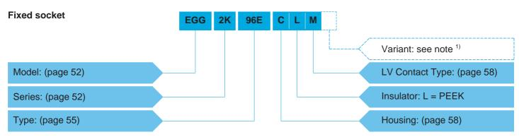
**EGG.2K.96E.CLM** = Fixed socket with key (G), 2K series, mixed type to accept take 1 F1 type fibre optic contact and 6 low voltage contacts, chrome-plated brass housing, PEEK insulator, 6 female crimp electrical contacts.
