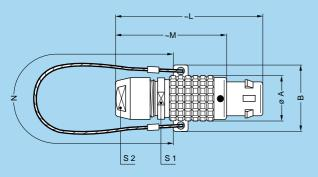
FNG Straight plug, key (G) or keys (A...L and R) and cable collet with lanyard release
