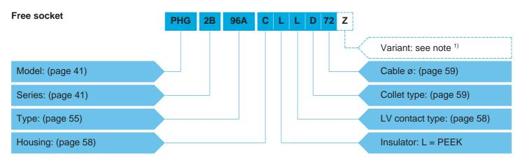
**PHG.2B.96A.CLLD72Z** = Free socket with key (G), 2B series, mixed type to accept 1 F1 fibre optic contact and 2 low voltage electrical contacts, chrome-plated brass housing, PEEK insulator, 2 female solder electrical contacts, type D collet system to suit a 7.2 mm diameter cable, and a nut for fitting a bend relief.
