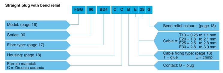
**FGG.00.BD4.CCBE25G** = Straight plug with key (G), 00 series for single-mode or multi-mode fibres, F4 fibre optic contact, ferrule hole diameter 128 μm, chrome-plated brass housing, zirconia ceramic ferrule, plug type contact, crimp type cable fixing for 2.5 to 2.8 mm diameter cable, and gray bend relief.
