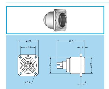
EBW.3K Fixed socket with front square flange (4 holes fixing), keys (W)
