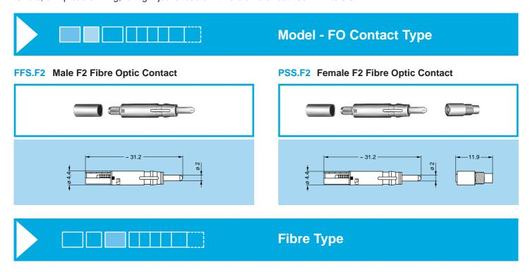
The choice of the ferrule hole diameter is dependent upon the fibre cladding size. LEMO offers a range of ferrule hole diameters to suit the users' specific requirements.
