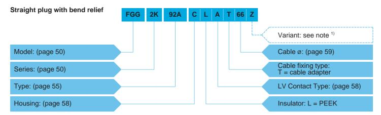
**FGG.2K.92A.CLAT66Z** = Straight plug with key (G), 2K series, mixed type to accept 1 F2 type fibre optic contact and 2 low voltage contacts, chrome-plated brass housing, PEEK insulator, 2 male solder electrical contacts, cable fixing type T for 6.5 mm diameter cable, and nut for fitting a bend relief.
