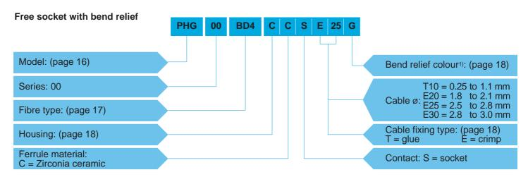
**PHG.00.BD4.CCSE25G** = Free socket with key (G), 00 series for single-mode or multi-mode fibres, F4 fibre optic contact, ferrule hole diameter 128  $\mu$ m, chrome-plated brass housing, zirconia ceramic ferrule, socket type contact, crimp type cable fixing for 2.5 to 2.8 mm diameter cable, and gray bend relief.
