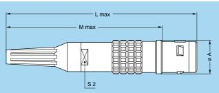
FGG Straight plug, key (G) or keys (A...F, L and R), cable adapter and nut for fitting a bend relief
