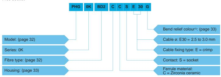
**PHG.0K.BD2.CCSE30G** = Free socket with key (G), 0K series, F2 fibre optic contact, ferrule hole  $\emptyset$  128  $\mu$ m, chrome-plated brass housing, zirconia ceramic ferrule, socket type contact, crimp type cable fixing for 2.5 to 3.0 mm diameter cable, and gray bend relief.
