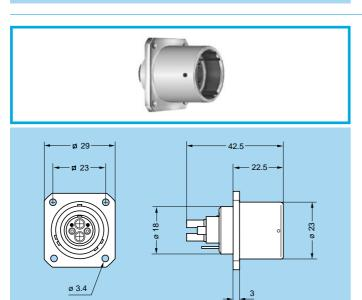
EDW.3K Fixed socket with rear square flange (4 holes fixing), keys (W), and earthing tag
