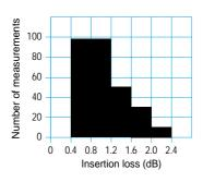
Mean = 1.13 dBTested at 850 nm Tested according to the standard IEC 61300-03-04, Insertion Method B. Fibre =  $200/230 \mu m$ Ferrule bore diameter = 235 µm
