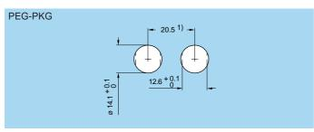
Note:  $^{1)}$  Minimum distance between two neighbouring components. Mounting nut torque: 5 Nm. The value shown above is the maximum torque for each connector type.
