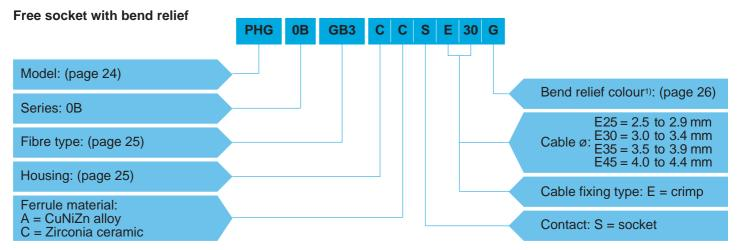
**PHG.0B.GB3.CCSE30G** = Free socket with key (G), 0B series, F3 fibre optic contact, ferrule hole diameter 235  $\mu$ m, chrome-plated brass housing, zirconia ceramic ferrule, socket type contact, crimp type cable fixing for 3.0 to 3.4 mm diameter cable, and gray bend relief.
