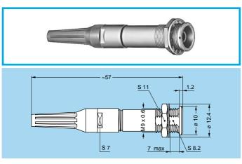
PFG.0B Fixed socket, with two nuts, key (G) or keys (A...F), with bend relief, (back panel mounting)
