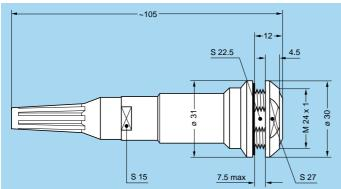
PEW.3K Fixed socket, nut fixing, keys (W), cable adapter, with bend relief (back panel mounting)
